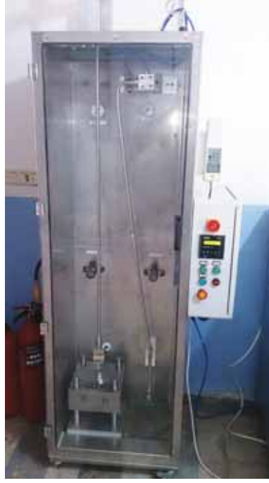
Spiral Gergi ve Mukavemet Testi Shower Hose Tension and Pressure Testing
