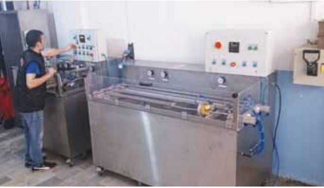
Spiral Su, Sıcaklık ve Burkulma Testi / Shower Hose Tension and Flowrate Testing
