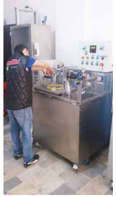
El Duşu Mukavemet ve Su Testi Shower Head Tension and Flowrate Testing
